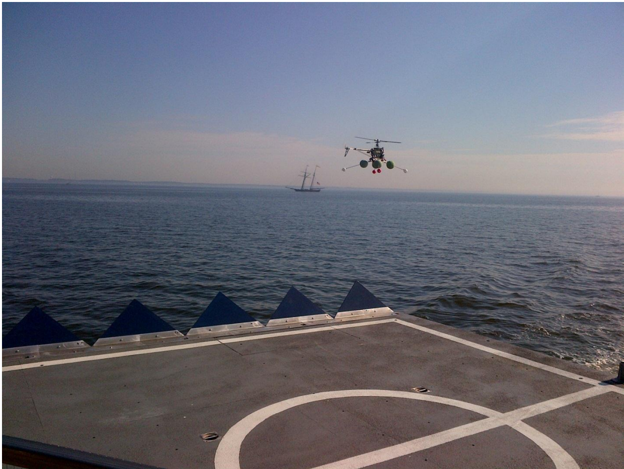
Figure 26. Flow control fences (blue wedges) added to the top, port and starboard sides of hangar structure and starboard side of flight deck.
