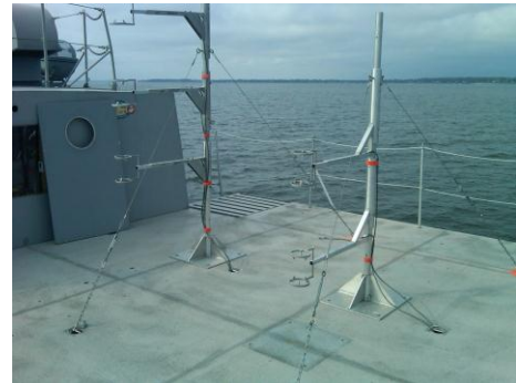
Figure 4. Ultrasonic anemometers installed on YP676 flight deck.
