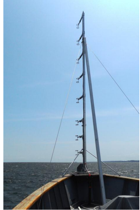
Figure 7. Bow anemometer array. Reference anemometer is third from bottom.
