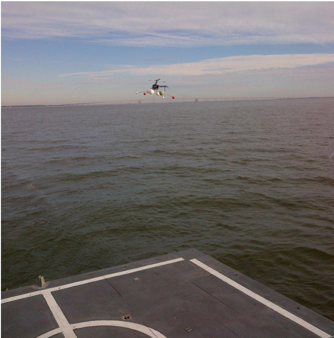
Figure 18. Radio controlled instrumented helicopter flying astern of YP676 in the Chesapeake Bay.
