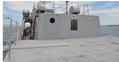
Figure 3. Detail of YP676 flight deck and hangar-like structure.
