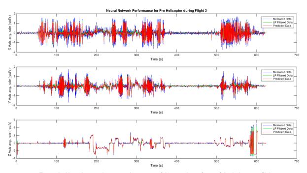
Figure 6. Neural network test results on one of the test data of one of the indoor test flight
