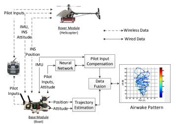
Figure 4. Schematics of proposed Telemetry System
