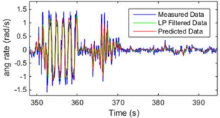
Figure 7: Prediction results for angular rates along x axis
