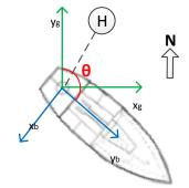
Figure 9. Coordinate system of the ship
