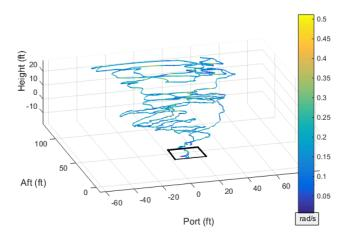
Figure 10. Isometric view of the ship air wake intensity plotted on the helicopter's trajectory.
