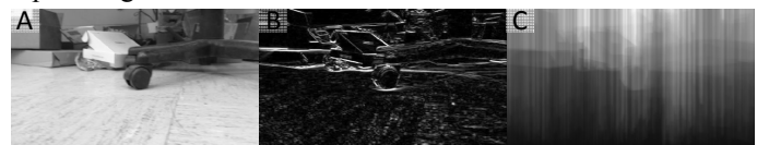
Figure 8. Floor boundary cue: (A) Input image (grayscale channel), (B) Horizontal edges, and (C) Cumulated edge map.
