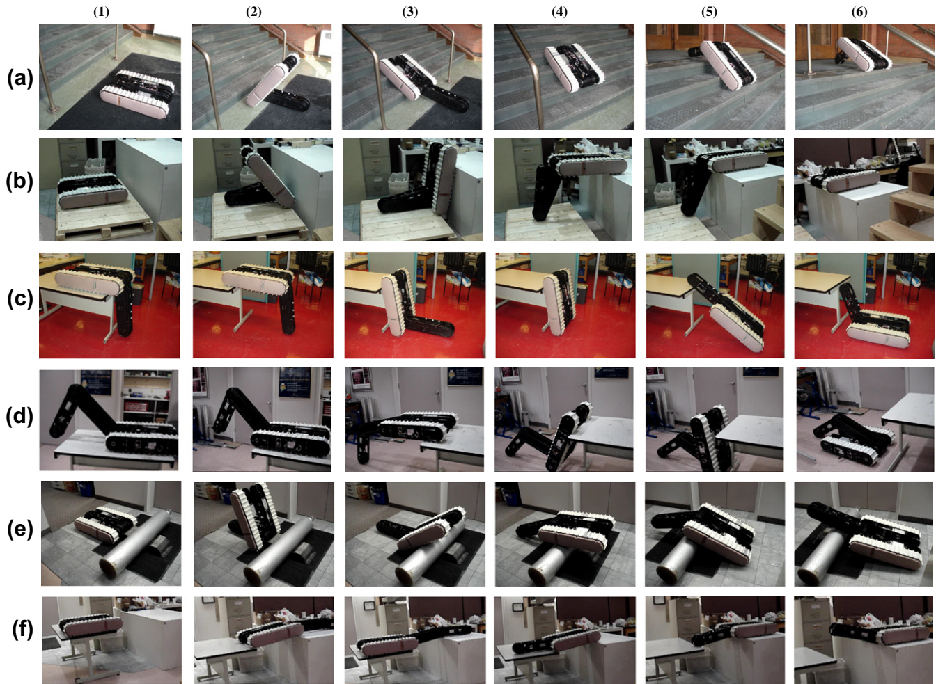
Fig. 16. Experimental results: (a) stair climbing; (b) step climbing with tracks; (c, and d) step descending; (e) surmounting tall cylindrical obstacles; (f) ditch crossing.
