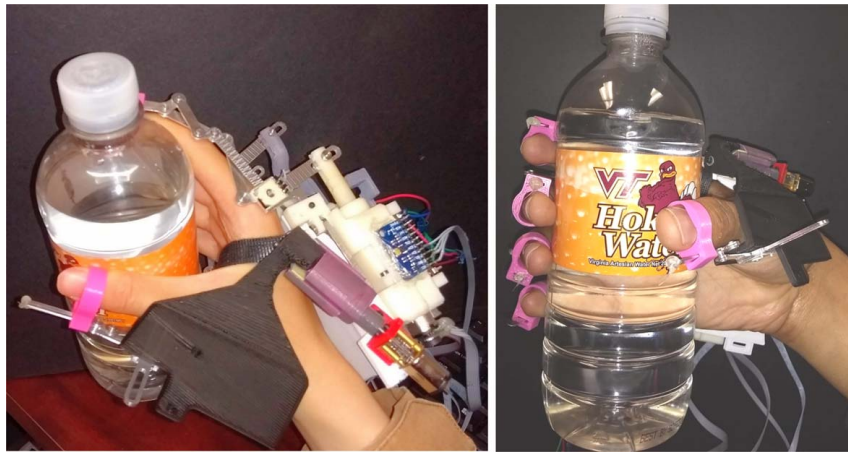
Fig. 20 Prototype glove shown here was used for testing the optimal force algorithm. The object in this case the water bottle is grasped and then the forces are applied as generated by the algorithm.
