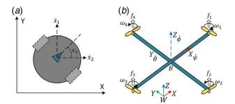
Fig. 1 Kinematic model of robot platforms
