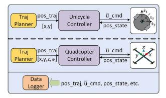
Fig. 3 Simulation system for the unicycle and the quadcopter
