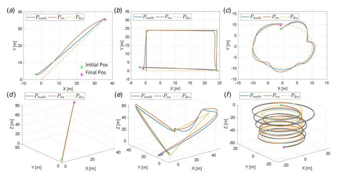
Fig. 4 Point-to-point, Square and Circle motion for (a)-(c) the unicycle and (d)-(f) the Quadcopter
